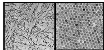
**Metal oxides (FeOx, CoO, CeO<sub>2</sub>, TiO<sub>2</sub>, CuO, ZnO):** Several synthetic routes available: decomposition of organo-metallic precursors in organic solvents, sol-gel processes, hydrothermal decomposition of metal salts, oxidation of metal nanoparticles, precipitation of metal salts in basic conditions, and even with mechanical milling and/or grinding.
