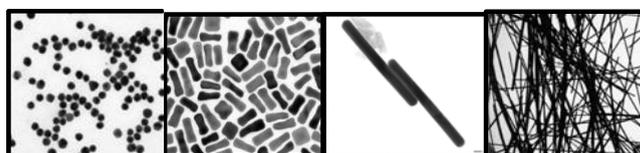
**Ag:** Preparation of Ag NPs in aqueous phase (citrate-reduction or NaBH<sub>4</sub>), using AgNO<sub>3</sub> in polar solvents. NPs from 10 nm to 80 nm are obtained. In organic solvents starting from AgNO<sub>3</sub> can narrow the size distribution and Ag NPs can later be transferred to water. Control of size and shape – nanospheres, nanocubes, nanorods and nanowires – is achieved using polyols and in the presence of polymeric stabilizers (PVP).
