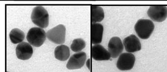
**Pt:** Pt NPs of different shape morphologies (cubic, polypod, cuboctahedrons and raspberries). Synthesis in an organic solvent using Pt(acac)<sub>2</sub>, oleylamine and/or 1,2 hexadecanediol. In aqueous solution the reduction of platinum salts with sodium citrate or NaBH<sub>4</sub> yields to Pt NPs of small size (2-3 nm).
