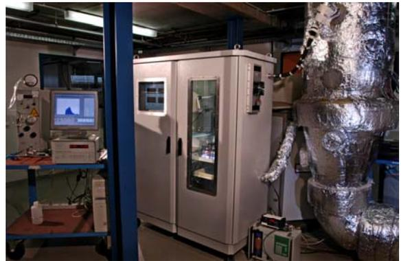
Photographs of the fully automated and temperature controlled prototype of the **Karlsruhe Exposure System** during an outside measurement of environmental aerosols (left) and at a technical plant (right).
