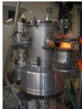
Atmospheric - PMS attached to a McKenna burner
