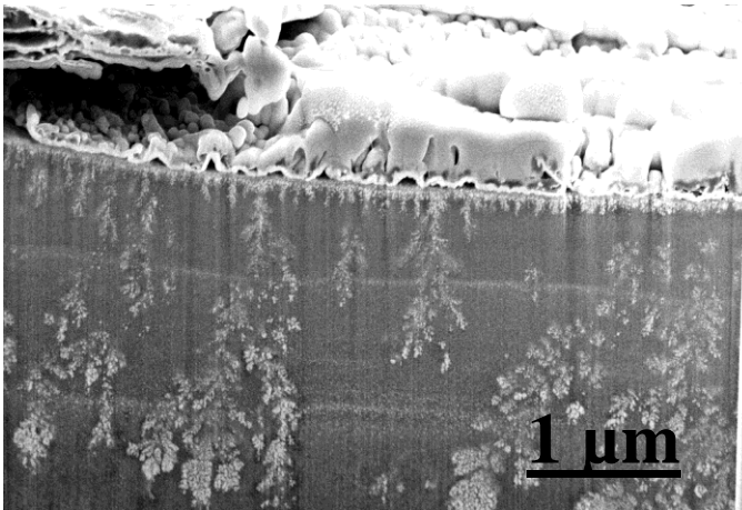
FIB cross section of buried silver nano-particles in a polymer host material. [A. Satti, Y.K. Gun'ko, TCD]
