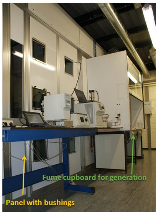
Figure 1: Indoor Nano Aerosol Exposure Test Chamber, (Left) Sidewall, and (Right) Floor Plan
